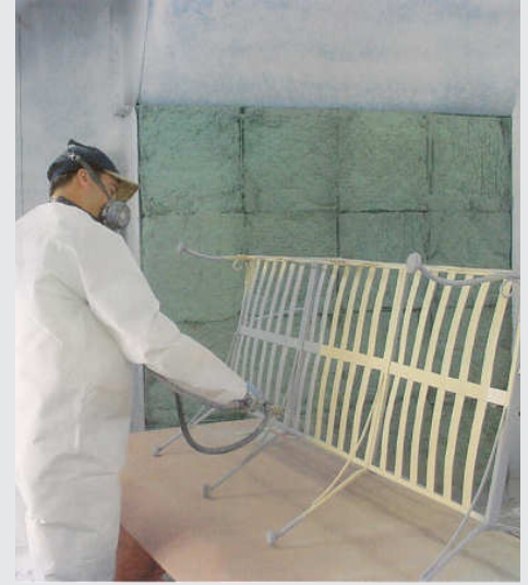
Figure 9.5-3 Spray Coating Operation 49
