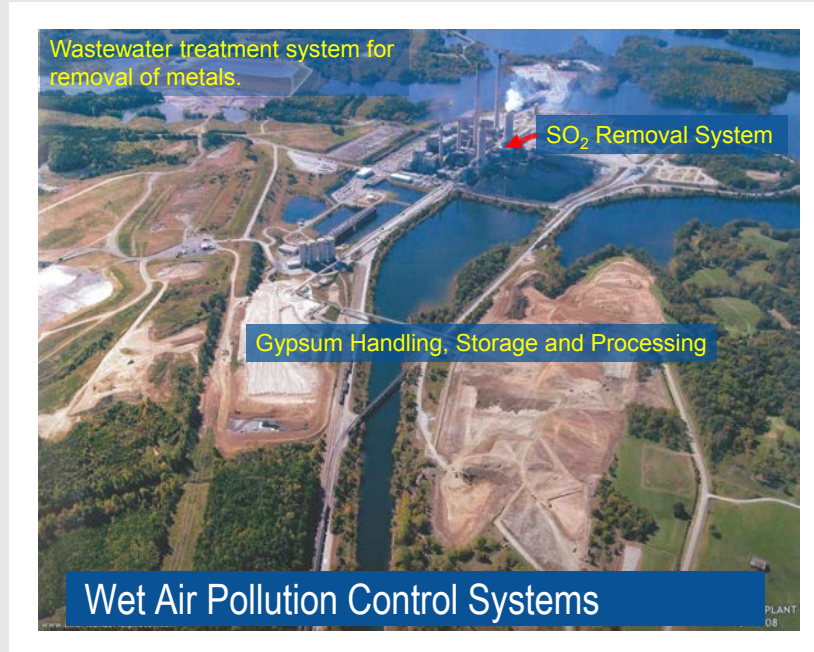
Figure 9.1-11 Typical Footprint of a Wet FGD System Producing High-quality Gypsum
